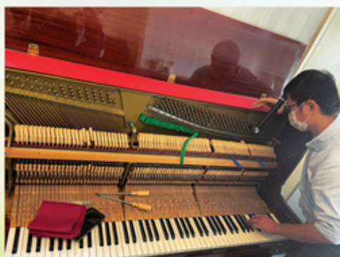
調音師進行鋼琴調音服務 The technician is tuning the piano
