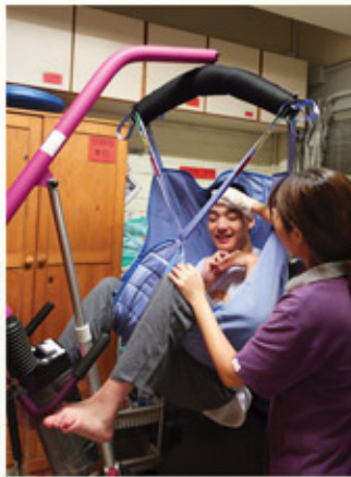
流動吊機讓宿生在轉移位置時更安全及舒適 The electric mobile hoist enables a more effective and safer way of transferring wheelchair-bound students
